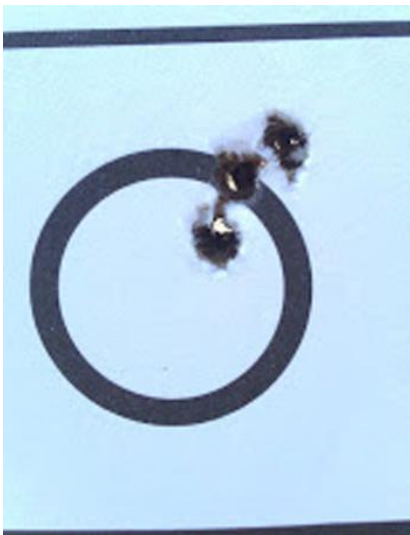
[SIZE="1"].46 MOA Group with a Cooper Model 21 .204 firing handloaded 39 grain Sierra Blitzking. [/SIZE]
