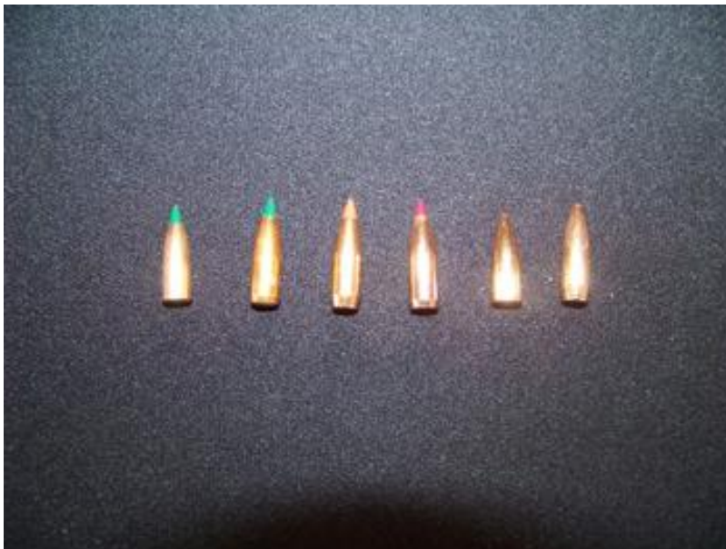
Twenty Cal bullets by increasing penetration. 32 BK, 39 BK, 40 V-max, 40 NOS BT, 35 Brgr, 40 Brgr
